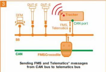
\* Telematics messages contain most important information on vehicle operation. FMS gateway gathers messages by scanning CAN bus.
